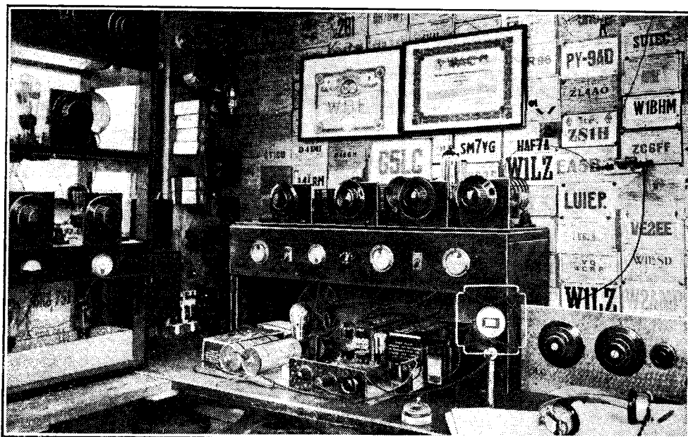
A COMPACT AMATEUR STATION. G5LC, East Molesey, Surrey, which is owned and operated by Mr. Leslie Cooper. The transmitter in the centre is a crystal oscillator, neutralised buffer amplifier, locked T.p.—T.g.rig for 20 and 40 metres. On the left is the 80 and 160 metres transmitter using a pentode crystal oscillator and power amplifier. The station has worked all continents and 52 countries.
