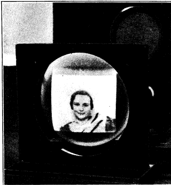
180-LINE IMAGE. An untouched picture of the lady announcer at Berlin "Post Office" station shown on the screen of an experimental equipment of Manfred von Ardenne, who is working in conjunction with the firm of C. Lorenz.
